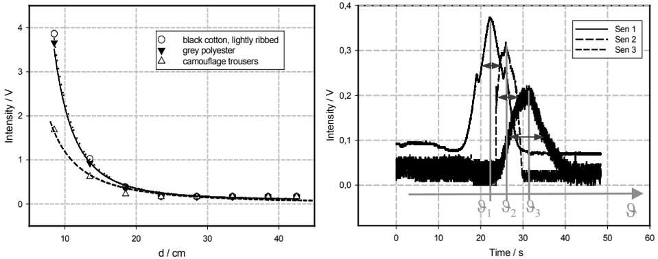
Figure 3: Intensities as a function of object distance from the light source for different materials (left) and as a function of the angles of incidence corresponding to the time instants in case of a reflector moving across the detector array with constant velocity (right)
