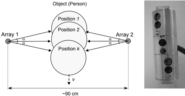
Figure 1: Basic configuration of the detector (top view) and view of a sensor array consisting of three emitter/receiver diode pairs
