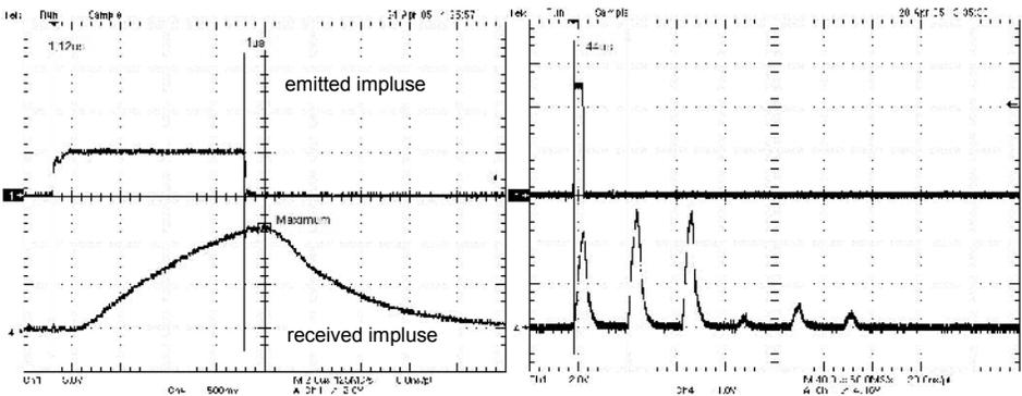
Figure 2: Transmitted pulse and received pulses for 1 sensor (left) and for 6 sensors (right).
