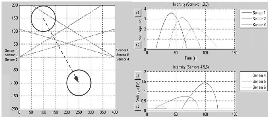
Figure 4: Trajectory of motion of a cylindrical object and light intensities reflected from the object's surface received at every sensor
