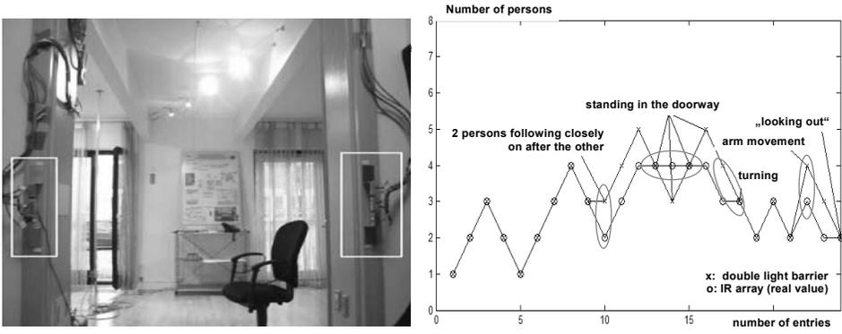
Figure 5: People counter mounted at a door and results compared with a double-beam light barrier
