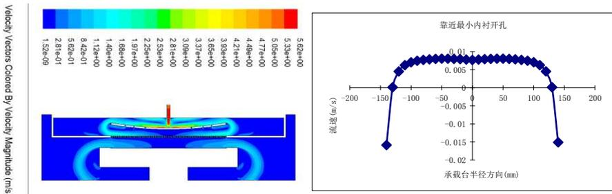
(a) velocity vector (b) velocity distribution near substrate
