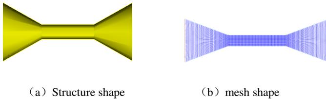
Figure 1: Shape of hole on the second showerhead
