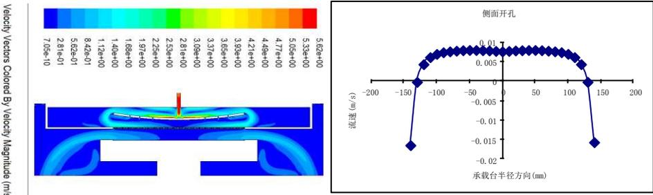
(a) velocity vector (b) velocity distribution near substrate
