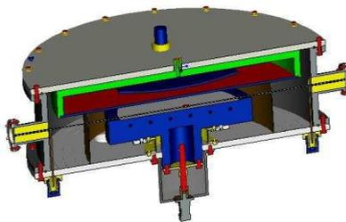
Figure 6: Structure of the processing chamber
