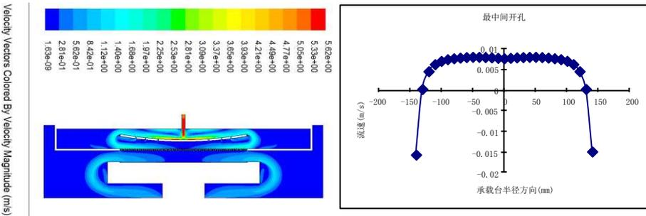
(a) velocity vector (b) velocity distribution near substrate
