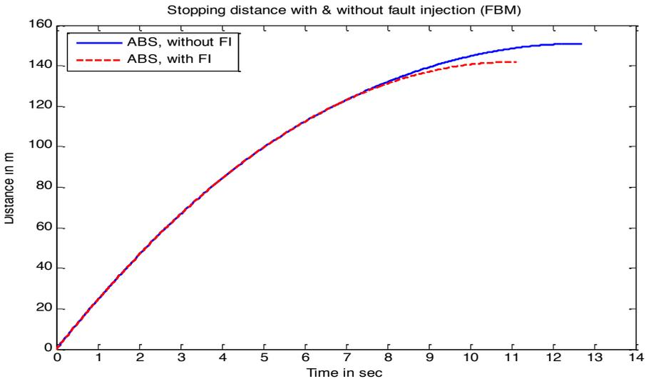
Figure 11: Using FBM shows for this system, the stopping distance would increase by approx. 6m under given fault conditions.
