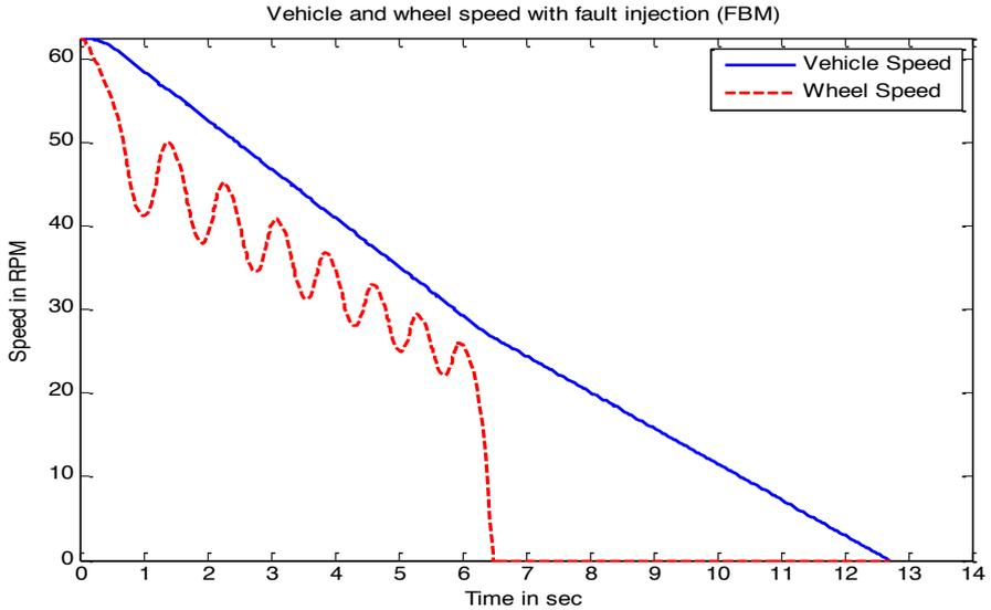
Figure 10: Using FBM shows wheel locking at  $t=6\text{sec}$ , time of fault injection.
