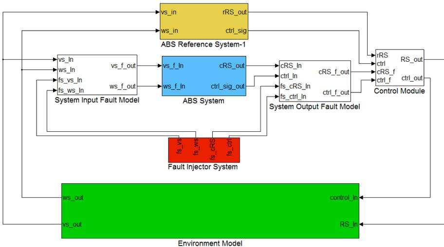
Figure 8: ABS system-environment model representation in Simulink with fault injector setup using FBM.
