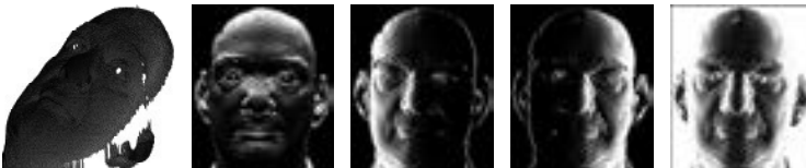
Figure 2: from the left to the right: the plotted raw-3D data (just for better imagination of the real face), the y -gradient, the x -gradient, the mirrored- x -gradient and a new developed gradient visualization named x -abs-gradient.
