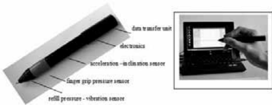
Figure 1: a view of the Biometric Smart Pen “BiSP” equipped with a diversity of sensors for monitoring handwriting movements on paper pad and in air.
