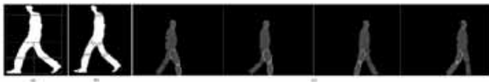
Figure 2: (a): body parts, (b): ellipse fitting model and (c) tracking of legs, blue ellipses for the leg closer to the camera
