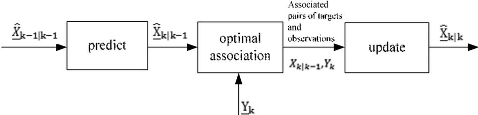
Figure 1: Block diagram for a multi-target estimation process
