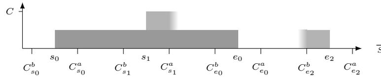
■ **Figure 2** Load profile for the **Cumulative** constraint with  $C = 2$  and  $\vec{S} = \{\alpha, s_0, s_1, e_0, e_2, \omega\}$ . Each activity has a load of 1, activity 0 ( $s_0, e_0$ ) is fully inserted (dark gray) and both activity 1 and 2 are partially inserted (light gray).  $e_1$  is considered to be inserted right after  $s_1$ , whose load only affects  $C_{s_1}^a$ . For activity 2,  $s_2$  is considered to be inserted before  $e_2$ , affecting the value  $C_{e_2}^b$ .
