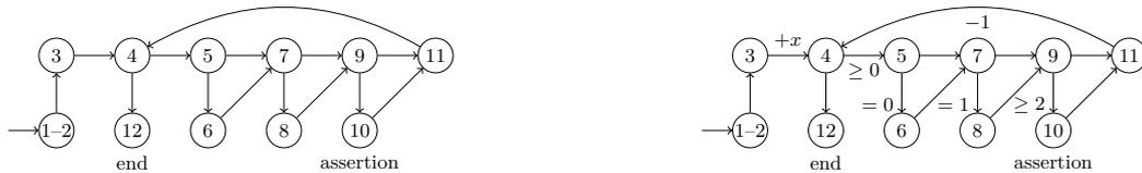
■ **Figure 1** On the left, the CFG with vertex labels corresponding to source code line numbers; on the right, the CFG extended by tracking the value of  $i$ .
