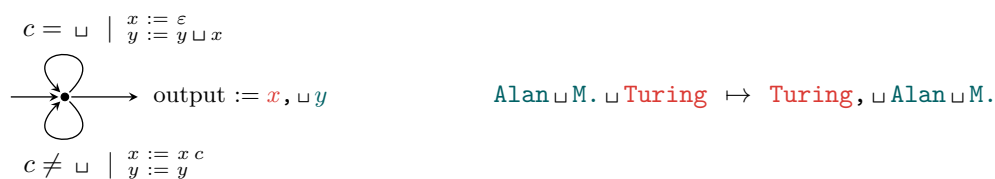
■ Figure 3 A DSST that updates two registers, named x, y , based on whether the input letter c is the blank space or not.
