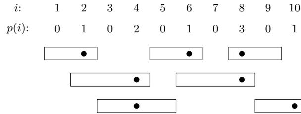
■ **Figure 3** Execution of Algorithm **Priority** on an instance with ten items and seven conflicts. The dots represent the items that were chosen by the algorithm. The computed solution is  $P = \{4, 8, 10\}$ , while the optimum is  $\{1, 3, 6, 9\}$ .
