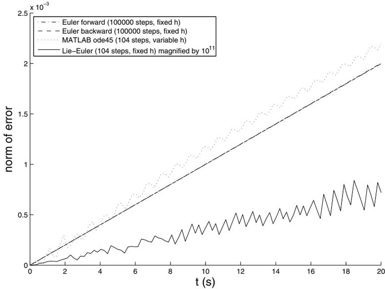
Figure 5: Comparison to the exact analytical solution on the equator of  $S^2$ . Note that the error of the Lie-Euler integrator is scaled by a factor of  $10^{11}$ . The error values of the two classic Euler schemes are almost indistinguishable.
