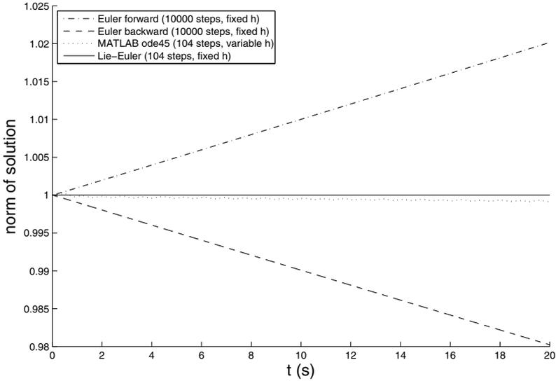
Figure 4: Deviation of trajectories from the configuration manifold  $S^2$  for the different integration schemes illustrated by the fact that  $\mathbf{x}(t) \in S^2 \Leftrightarrow \|\mathbf{x}(t)\| = 1$ .
