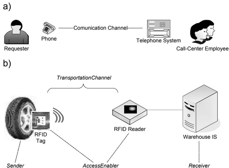
Figure 1: Examples for Transportation Channels
