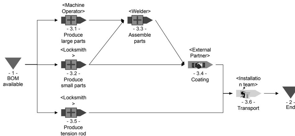
Figure 3: Sample Production Process (source: [Di01], p. 36)
