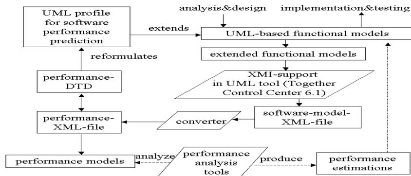
Figure 1: Framework for predicting software performance during analysis and design
