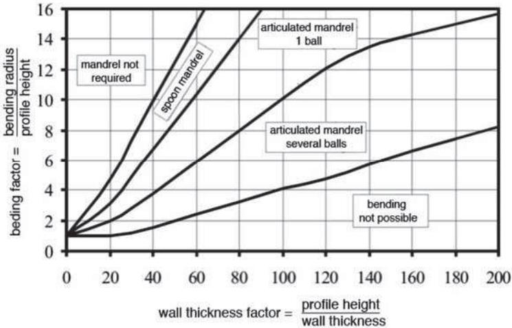
Fig. 2: Bending diagram for mandrel selection [VDI3430]
