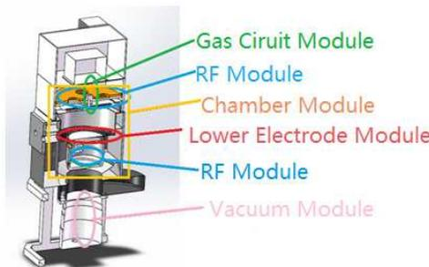
Figure 4: Experiment platform module
