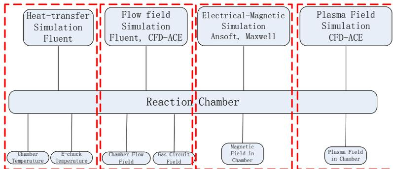
Figure 6: Simulation platform system
