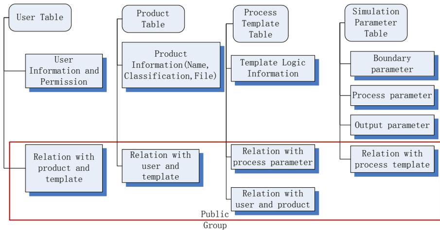
Figure 2: Database structure
