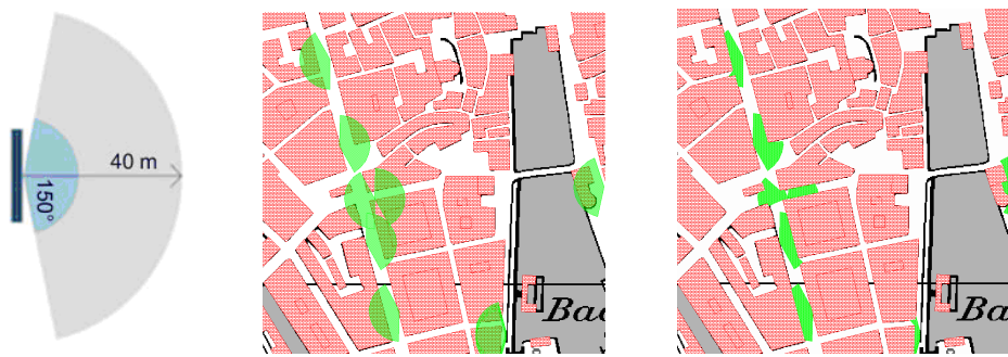
Figure 2: Standardized visibility area of a panel (left), overlay of visibility areas and building layer (middle) and visibility areas after intersection with building layer (right)
