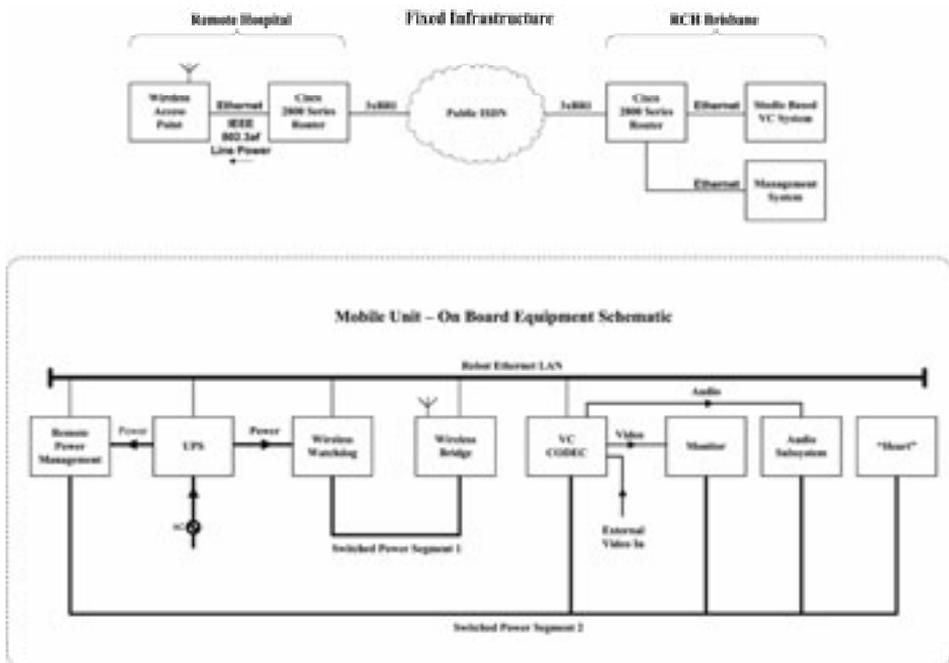
Fig. 3.4 – Second generation telepaediatric robot and related fixed infrastructure
