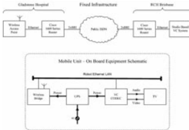
Fig. 3.3 – Prototype telepaediatric robot and related fixed infrastructure
