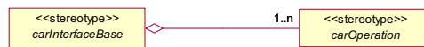
Figure 4: Extensions of the UML metamodel: each interface class contains at least one operation.
